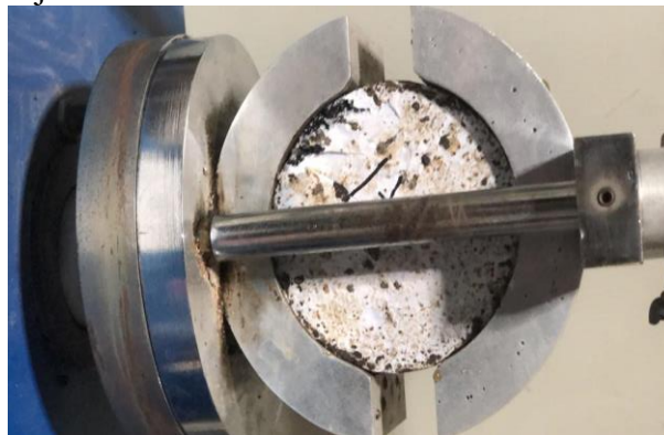
Gambar 3.30 Sampel Uji Marshall LASTON AC-WC
