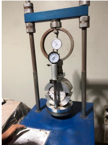
Gambar 3.29 Alat Marshall Test
