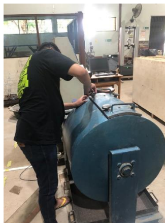
Gambar 3.7 Pengujian Los Angeles Abration
