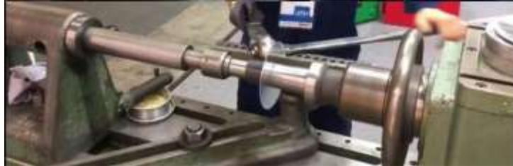
**Gambar 2.17.** Metal spinning manual
