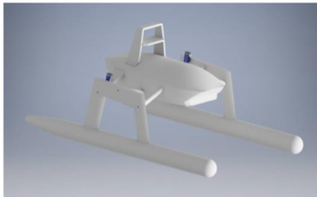
Figure 1: The hull form of the SWATH-ASV
