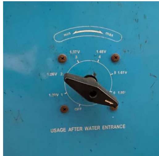
Gambar 3. 8 Adjustment of welding voltage
