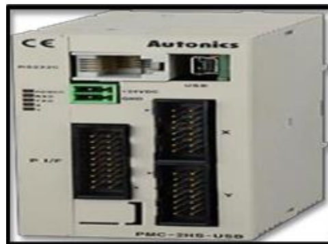
Gambar 3.7 Motion Controller PMC-2HS-USB
