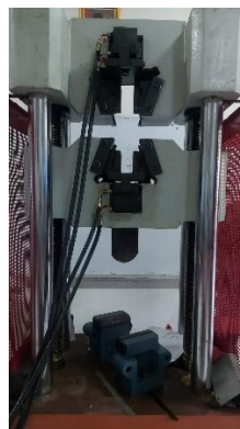
Gambar 3.8 Universal Testing Machine
