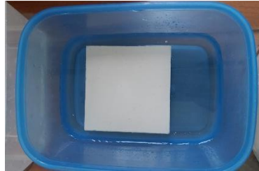
Gambar 3.29 Perendaman Sampel 10 \times 10 \times 1 \text{ cm}^3
