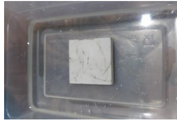
Gambar 3.31 Perendaman Sampel 5 \times 5 \times 1 \text{ cm}^3
