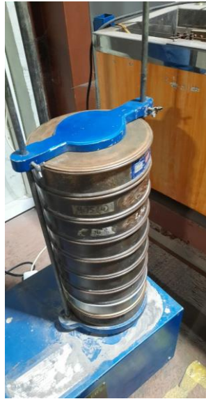
Gambar 3. 17 Proses Uji Sieve Shaker
