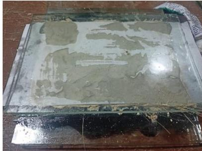
**Gambar 3. 27** Proses Penutupan Adonan Gypsum
