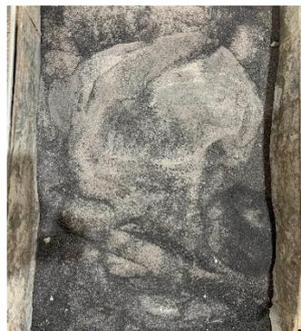
**Gambar 2. 8** Abu Cangkang Kelapa Sawit (POFA)
