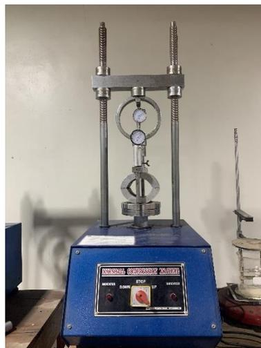
**Gambar 2. 6** Alat *Marshall Test*
