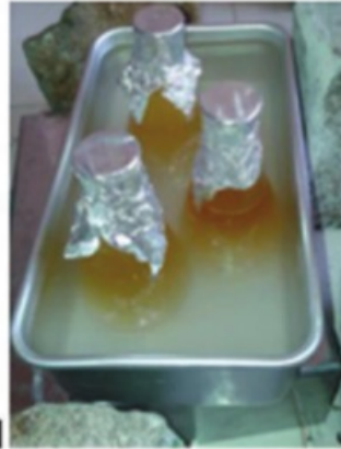
FIGURE 2. Transesterification CPO, Jatropha oil and Methanol on ultrasonic generator
