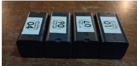
Gambar I-9 Baterai Total Station reflectorless dan GNSS Topcon Hiper II
