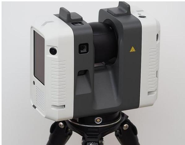
**Gambar I-3.** 3D *Laser scanner* RTC360 (Kurkela, 2021).
