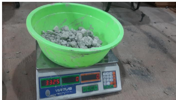
Gambar 4.15 Timbang Limbah Beton
