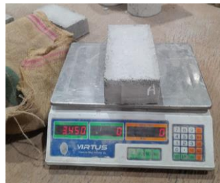
Gambar 3. 49 Penimbangan benda uji paving block
