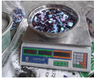
Gambar 3. 36 Proses penimbangan microfiber
