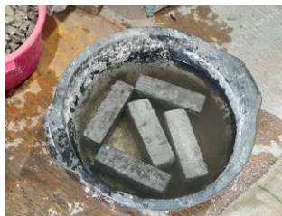
Gambar 3. 52 Perendaman benda uji paving block
