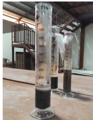
Gambar 3. 33 Hasil pengujian kadar lumpur metode cucian
