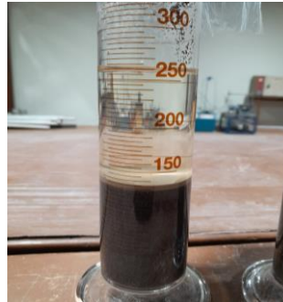
Gambar 3. 27 Hasil pengujian kadar organik
