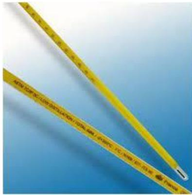
Gambar 3.6 Termometer air raksa ASTM 12C
