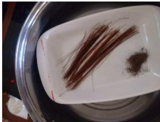
Gambar 3.39. Proses steaming serat
