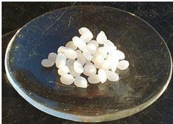
Gambar 3.16. Alkali (NaOH)
