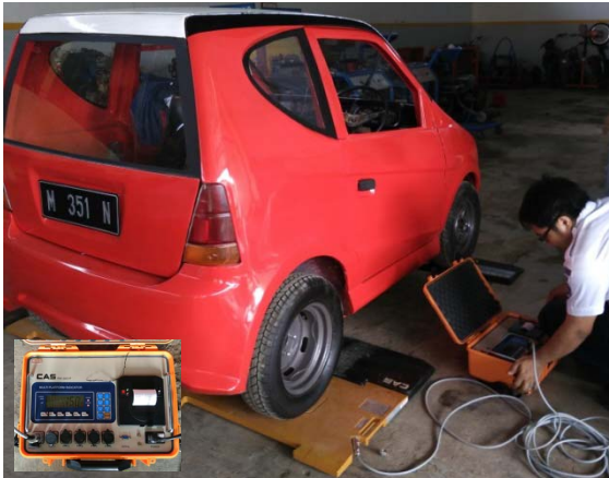
Fig. 9. The curb weight measurement
