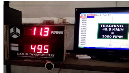
Fig. 11. Test calibration process, linear wheel speed display (left), power car torque and graphic display (right)
