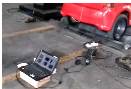
Fig. 13. SOC testing using coulomb counting method
