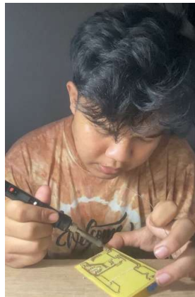
Gambar 4. 2 Proses Solder PCB
