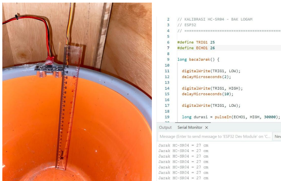
Gambar 4. 33 Kalibrasi Sensor HC-SR04 Bak Logam
