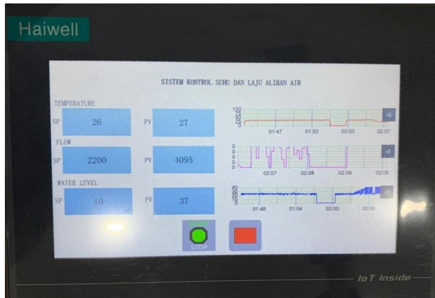
Gambar 4. 23 Tampilan Antarmuka Haiwell Cloud SCADA Saat Monitoring Sistem
