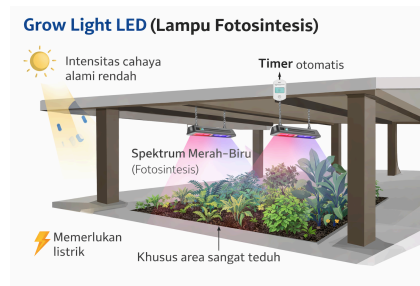
Gambar 2.9 Diagram Konsep Grow Light LED
