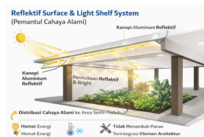
Gambar 2.10 Diagram Konsep Reflektif Surface & Light Shelf System
