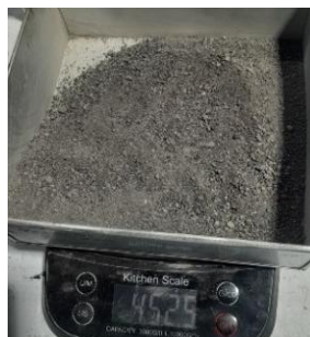
Gambar 3.33. Penimbangan Agregat Halus Hasil Kadar Lumpur
