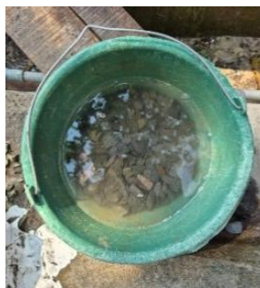
Gambar 3.49. Pencucian Agregat Kasar
