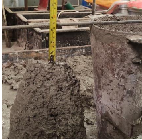
Gambar 4.3. Hasil Uji Slump Beton Serat
