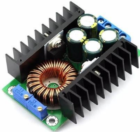
Gambar 2. 4 Step-Down Converter 300W
