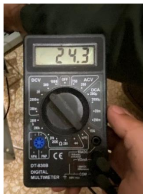
Gambar 4. 1. Tegangan Com PLC
