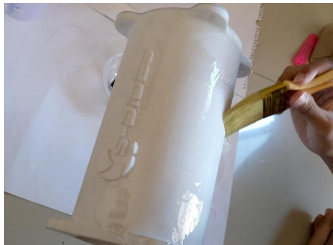
Gambar 4. 3 Proses Pelapisan Resin Epoxy
