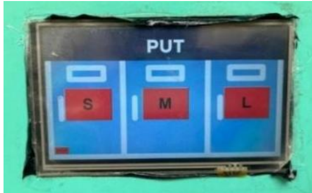
Gambar 4. 11 Tampilan HMI Mode Penyimpanan ( Put )
