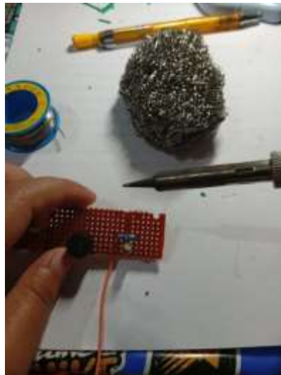
Gambar 4.6. Proses Pemasangan LED dan Buzzer
