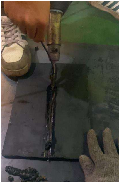
Gambar 4. 11 Proses Pengelasan Root
