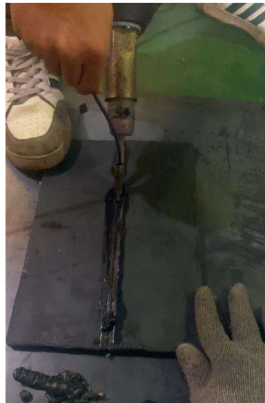
Gambar 4. 11 Proses Pengelasan Root
