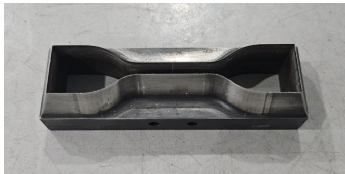
Gambar 4.2 Dies tipe C ASTM D412
