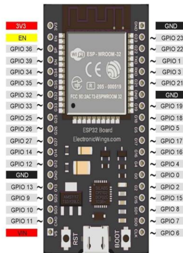
Gambar 2. 1 Pin ESP32
