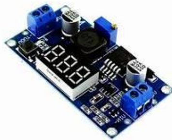
Gambar 2. 2 Step Down LM2956
