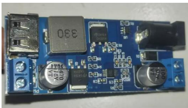
Gambar 2.15 Modul XY3606 DC Converter
