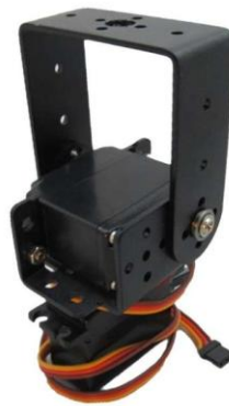
Gambar 2.6. Modul Pan-Tilt Servo [21]
