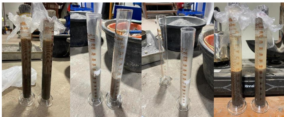
Gambar 3. 8 Pengujian Kadar Lumpur
