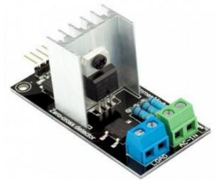
Gambar 2. 12 Modul AC Light Dimmer
