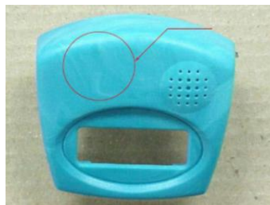
Gambar 2. 14 Cacat colour streak (Sumber: https://www.nexpcb.com )
