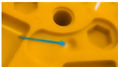
Gambar 2. 10 Cacat sink mark (sumber: https://prototool.com )
