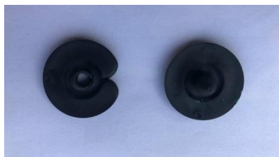
Gambar 2. 8 Cacat short shot (Sumber: https://www.topgrid.co )
