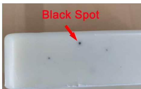
Gambar 2. 12 Cacat black spot (sumber: https://www.plasticmoulds.net ).
