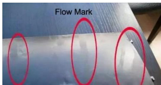
Gambar 2. 11 Cacat flow mark (Sumber: https://gudmould.wordpress.com )
