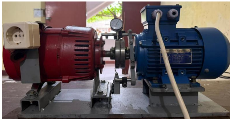
Gambar 4. 1 Hasil fabrikasi simulator shaft alignment
