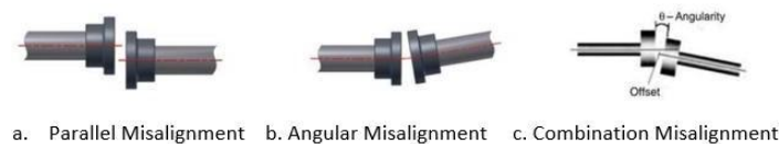
Gambar 2. 18 Macam - macam misalignment
