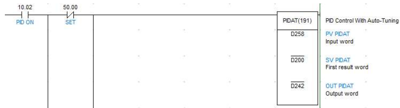
Gambar 4. 23 Program PIDAT PLC
