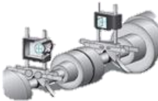
Gambar 2. 16 Shaft alignment metode laser
