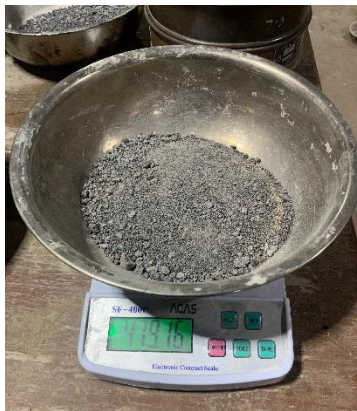
Gambar 3. 18 Menimbang Pasir Kering Oven
