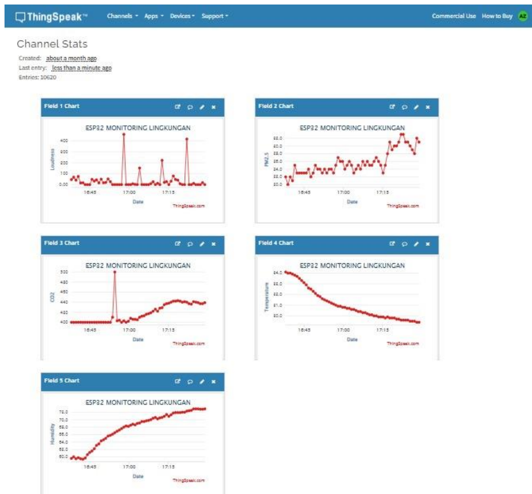
Gambar 5. 8 Tampilan Dashboard Sistem Monitoring di ThingSpeak
