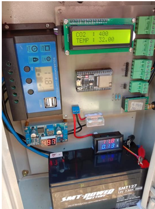
Gambar 4. 5 Hasil Perakitan Panel Box Transmitter
