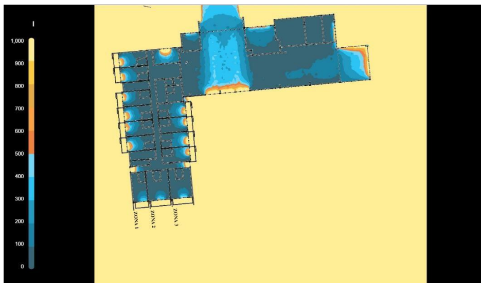
Gambar IV.133 Hasil Simulasi Fasad Overhang Sunshading Lantai 6 Jam 15.00
