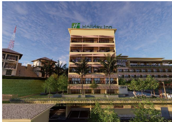
Gambar IV.107 Hasil Redesain Fasad Overhang Sunshading
