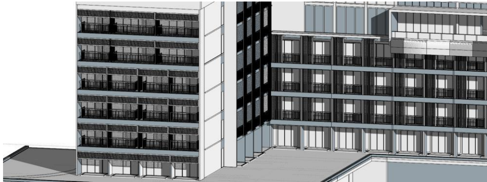
Gambar IV.109 Shading hasil redesign pukul 09.00
