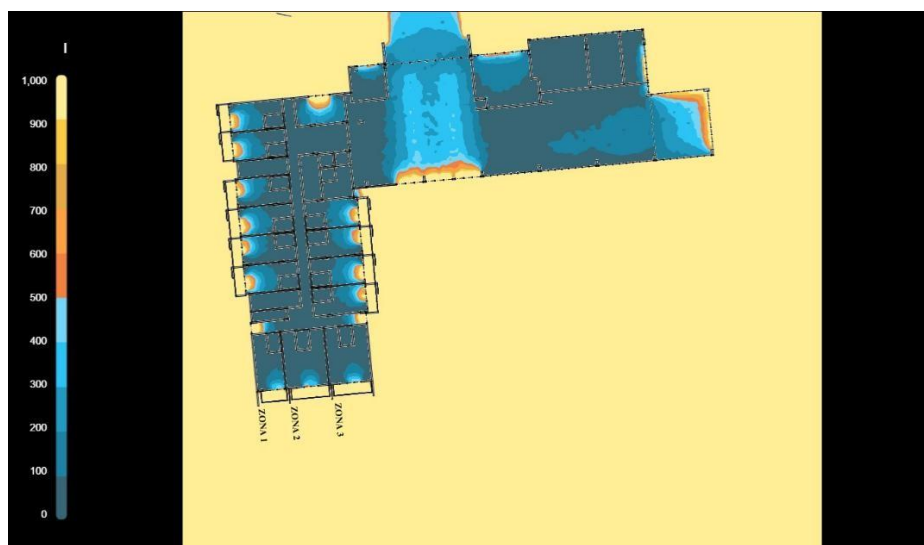
Gambar IV.131 Hasil Simulasi Fasad Overhang Sunshading Lantai 6 Jam 09.00
