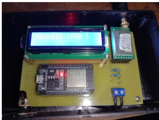
Gambar 4. 11 Hasil Perakitan Box Receiver
