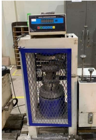
Gambar 3. 9 Digital compression machine
