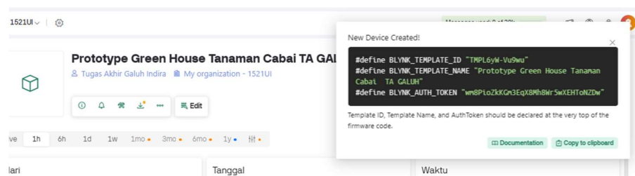
Gambar 4. 49 Integrasi Device ESP32 Blynk
