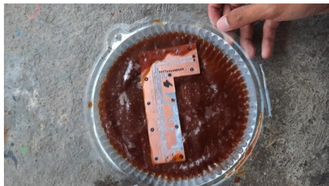
Gambar 4-11 Proses Etching PCB
