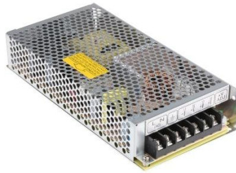
Gambar 2. 5 Power Supply Switching
