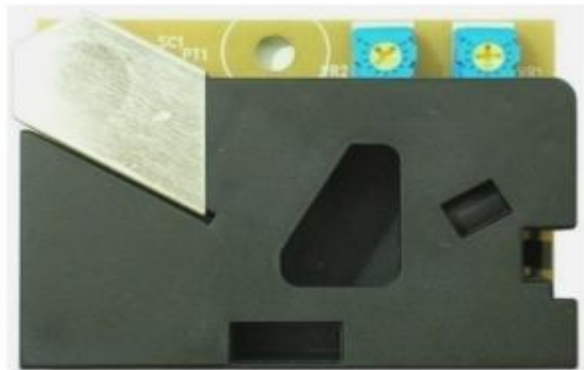
Gambar 2. 5 Sensor DSM 501A[16]
